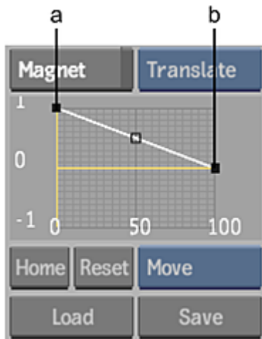
(a) Point representing effect at the Magnet's centre (b) Point representing effect at the Magnet's perimeter
