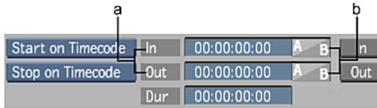
(a) In and Out timecode fields (b) 2:3 In and Out pulldown display
